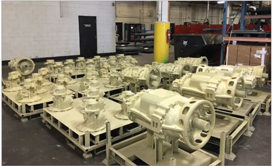
Powder coated air compressor airend housings ready for the assembly line.
